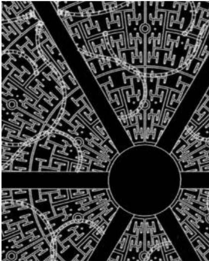
From an engineering point of view, another unusual characteristic is that the devices exhibit an invariance to scaling. Larger or smaller devices can be designed by adding or subtracting bifurcations while the symmetry of the device is maintained. This overcomes scale-up problems often encountered in taking a process from pilot to full scale operation. We have constructed functional surface distributors ranging in diameter from a few cm to 6.7 meter.
