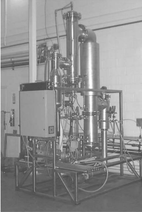
Peripheral pilot equipment, such as the rising film evaporator to the left, support pilot testing and provide production of large enough amounts of separated products for thorough customer evaluation or subsequent processing.
