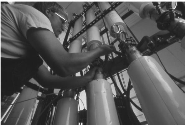
ARi operates several SMB pilot plants for evaluation of new applications and for determining customer separation and scale-up requirements. Six pilot simulated moving bed chromatography systems, all computer controlled, are available. The pilot plants are capable of evaluating a wide variety of feed materials including corrosive chemical mixtures.
