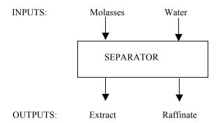
The feed materials consist of only molasses and water. Extract contains the recovered sucrose at high purity. This material is usually recycled in some way to the factory for eventual crystallization. The raffinate contains the molasses non-sugar and some sucrose. It is usually brixed up and used as a feed supplement or pulp additive.
