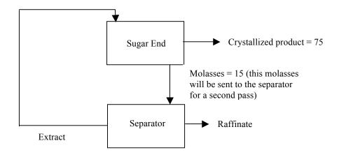
It is important to note that of the 100 units of sucrose entering the separator, only 75% was recovered as product. Additional labeled sucrose can be recovered by sending the 15 molasses units again into the separator—sugar end, separator—sugar end, etc. ad infinitum.
