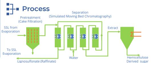
Following successful batch chromatography of SSL at laboratory scale an SMBC test was carried out on a 4 column pilot ARi SMBC system with Mitsubishi 530 cation resin in the magnesium form. The pulping waste side stream SSL was upgraded by evaporation, cake filtration and ARi Simulated Moving Bed Chromatography and the subsequent sugar rich extract from SMBC was concentrated to a dissolved solids of 60% to improve stability during storage and transport.
